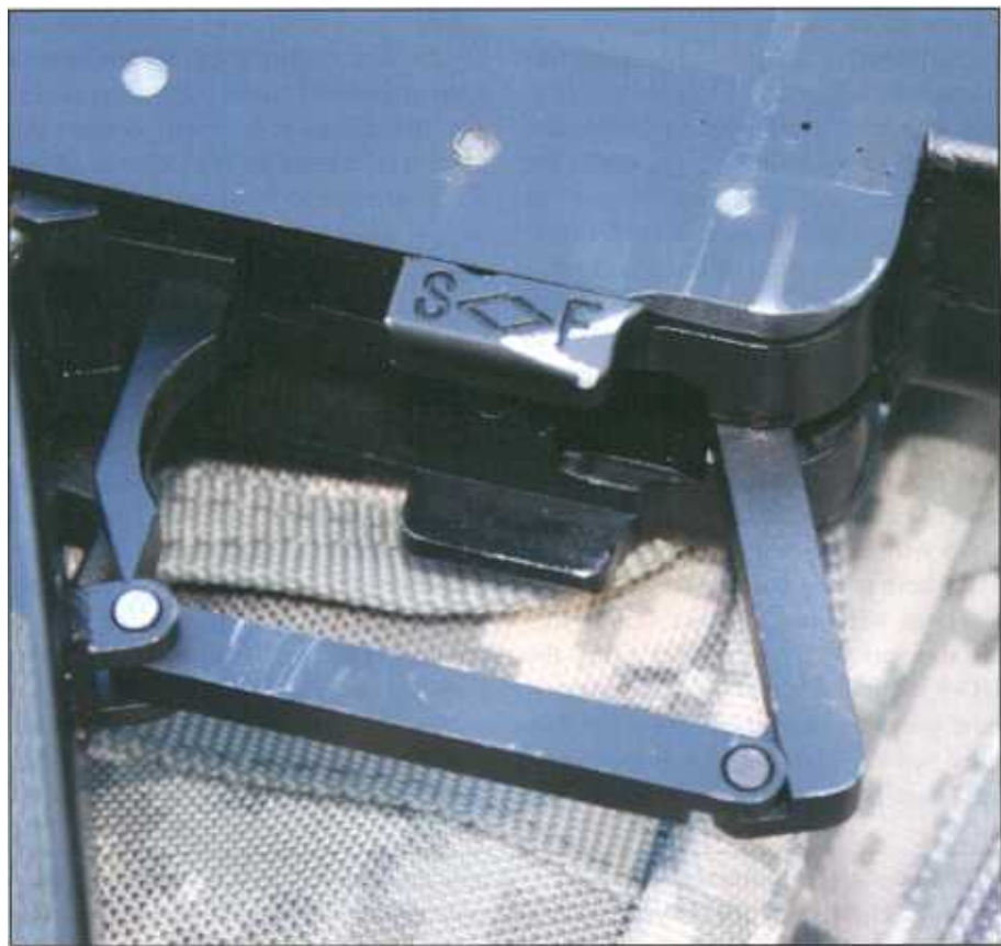
Above: The trigger-guard folds forward during closing as illustrated here. This complex design even includes a trigger that also folds forward allowing the mag-well to rest parallel to the barrel when closed.
